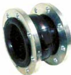
Flanges in galvanized steel. Elastic material: Polychloroprene. Maximum temperature: 95° C. Nominal pressure: 10 kg/cm<sup>2</sup> (PN/10).
