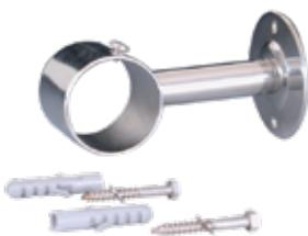
Made of AISI-316L polished stainless steel for Ø 43 mm handrails. Supplied with screws, gasket and wall plugs.
