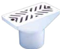
To be glued to a Ø 63 mm pipe. Body and grille in ABS plastic, screws in stainless steel. Application on wall. Its characteristics make this nozzle particularly suitable for overflow channels. Maximum flow rate: 4.5 m<sup>3</sup>/h.
