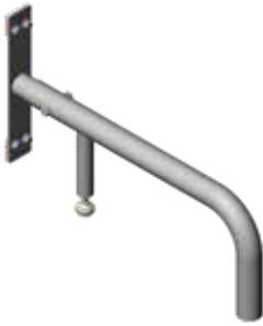
AISI-316 stainless steel ((for coupling to 00141 and 00142 fasteners, not included). State H and L dimensions and type of overflow channel when placing an order. A minimum of two units are required for each turning panel.
