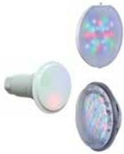
DMX lamps are powered at 12VAC. Must always work with DMX slave controller 41107 and a DMX master controller (for example the controller 74099).
