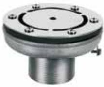
2" external thread. Made of AISI-316L stainless steel. Can be fitted in concrete and prefabricated pools. The water flow can be adjusted by loosening or tightening the central screw. Max. recommended flow rate complaint with standard EN 13451-3: 14 m<sup>3</sup>/h.
