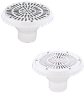
Made of white ABS plastic. Suction. Flow rate adjusted by turning the grille. Suction surface area: 0.015 m<sup>2</sup>. Outer Ø 295 mm wall. Flow rate (0.4 m/s) 20 m<sup>3</sup>/h. Max. recommended flow rate compliant with standard EN 13451-1: 26 m<sup>3</sup>/h (0.5 m/s).
