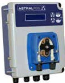
Automation flocculant dosing adjustable flow water pools. Includes: adjustable pump from 151 cm<sup>3</sup>/h until 1.5 l/h, injector valve, bottom filter, suction and return tube.
