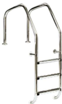
Ladder width 500 mm Ø 43 mm handrail, non-slip surface stainless treads, bright satin finish, anchoring fixtures for connection to the equipotential circuit and removable anchoring with plate for fastening to wall. AISI-316L handrail and steps.
