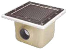
Made of fibreglass-reinforced polyester. With a gelcoat finish. Comes with gaskets, flange and screws. Holes < 8 mm. Outlet connection to be glued. With optional hydrostatic valve. Maximum recommended flow rate with stainless steel grille: 27 m<sup>3</sup>/h (0,5 m/s). Maximum recommended flow rate with ABS grille: 37 m<sup>3</sup>/h (0,5 m/s).
