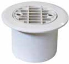
Return inlet for large flow rates that can also be used as a suction nozzle. Maximum suction flow rate of 30m<sup>3</sup>/h for a maximum flow rate speed of 4 m/s. Maximum suction flow rate of 5 m<sup>3</sup>/h for a maximum flow rate speed of 0.5 m/s. PVC body. Connection for Ø 75 or Ø 90mm pipe. Inlets can be installed into bushing 43590. Grille can be adjusted in any direction.
