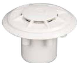
Adjustable pool floor return inlet for liner pools. Designed to be glued to the inside of PN6 and PN10 piping. Made of white ABS, with self-tapping screws or with metal inserts. Plastic or stainless steel flange, depending on the model. Maximum flow rate: 9.5 m<sup>3</sup>/h.
