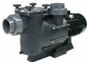
3000 rpm plastic centrifugal electric pumps with prefilter for pools, perfect for large, low-pressure flow rates. Prefilter with transparent lid and wishbone closure; easy access. Pump bodies and prefilter manufactured in fibreglass-reinforced polypropylene. Plastic turbine. Pump shaft and prefilter basket in stainless steel. Motors with 3000 rpm IP-55 protection at 230/400 V or 400/690 V and 50 Hz. From 4 HP to 12.5 HP.
