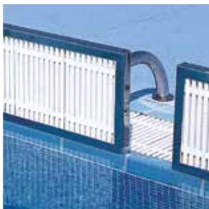
In AISI-316 stainless steel with plastic lattice screen. Height 300 mm. Fixing support (00139) is not included
