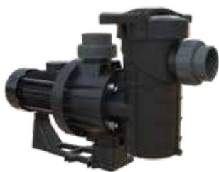
Pump body and supports in plastic, AISI-316 stainless steel motor shaft with double insulation. Motor has IP-55 protection rating. Prefilter basket with a capacity of 8 litres. Transparent prefilter lid.
