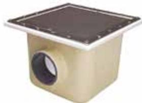
With a gelcoat finish. Grille in AISI-316L stainless steel. Comes with gaskets, flanges and screws. Holes < 8 mm. Outlet connection to be glued. Maximum recommended flow rate with stainless steel grille: 114 m<sup>3</sup>/h (0,5 m/s). Maximum recommended flow rate with ABS grille: 86 m<sup>3</sup>/h (0,5 m/s). With optional hydrostatic valve.
