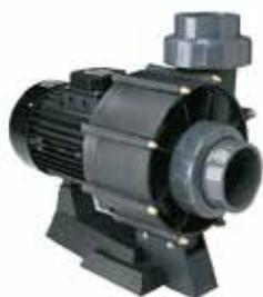
3000 rpm plastic centrifugal electric pumps with no prefilter for pools, perfect for large, low-pressure flow rates. Pump bodies manufactured in fibreglass-reinforced polypropylene. Plastic turbine. Stainless steel pump shaft. Motors with 3000 rpm IP-55 protection at 230/400 V or 400/690 V and 50Hz. From 7.5 HP to 12.5 HP.
