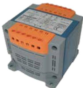
Single-phase Safety Transformers, especially designed for use in aquatic installations like pools or fountains. With the protection degree IP20 or more, primary of 230V AC and secondary of 12-13-14V AC.
