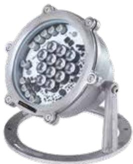
High-resistance projector, made with stainless steel. It is ideal for ornamental fountains and water jets. It should be installed completely submerged in water. It is provided with screws and studs for fitting. Possibility of intensive, intermediate or extensive lens.
