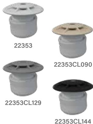
Swivel body in PVC. Cover in ABS. Adjuster screw in POM. Maximum flow rate of 10 m<sup>3</sup>/h. Fits to Ø 75 mm piping and wall conduit with code number 21248.
